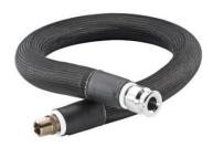
¾" ID Triple Insulated Flexible Hose has Welded-on S.S. Beaded Pipe Fitting for Connection to Reactor Inlet/Outlet. Uses CG-1968-69, 1 ½" BP Coupling (Sold Separately). Opposite End has ¾" Male NPT for Connection to Manifold Block.
